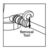
Step 1: Snap the removal tool over the pipe and align next to the fitting.
