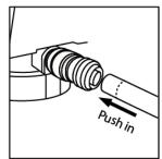
Step 3: Insert the pipe into the fitting.
