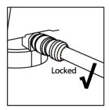
Step 4: Check the insertion depth mark.
