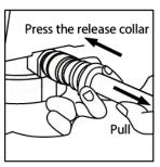
Step 2: Firmly push the removal tool over the collar of the fitting.
