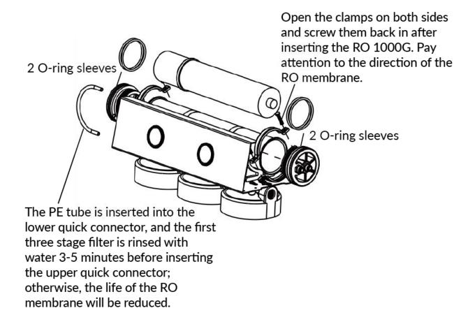
Figure 6. Machine Head Assembling
