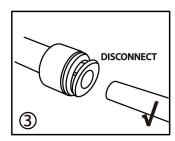
Figure 7. How to Install and Disconnect 1/4" and 3/8" Quick Fitting
