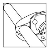
Step 1: Make a clean and square cut with a pipe cutter.
