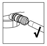
Step 3: Pull the pipe out of the fitting.
