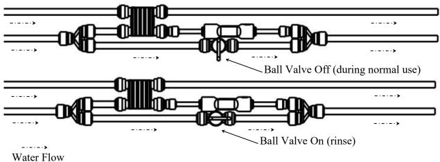
Figure 11. Valve Position
