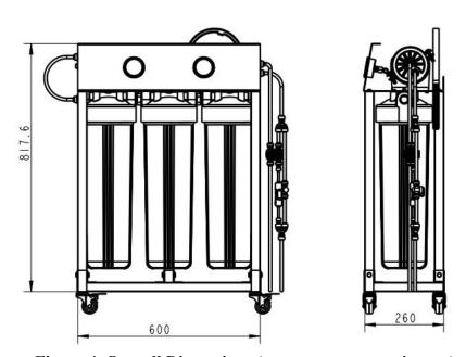
Figure 4. Overall Dimensions (measurements are in mm)
