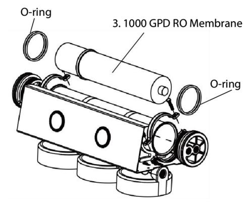
Figure 2. Machine Head
