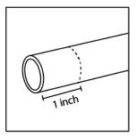
Step 2: Mark the pipe with 1 inch insertion depth.
