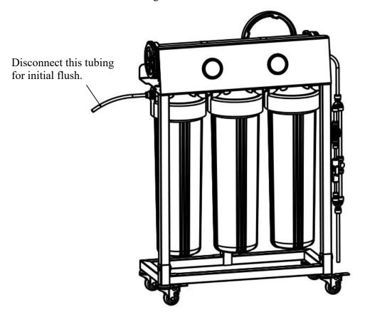
Figure 10. Flushing the System
