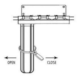
Figure 12. How to Use the Housing Wrench
