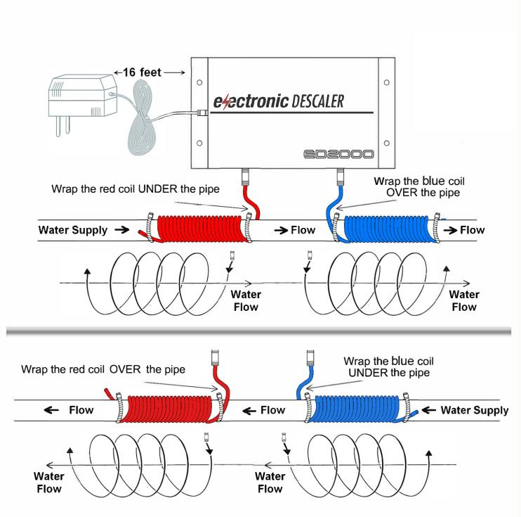
Wrap the full length of each coil around the pipe in their respective directions. Make sure the coils are wrapped snug against each other, leaving no space between the coils on each wrap.
