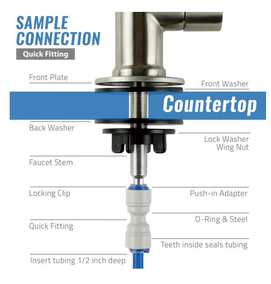
2. Slide the front plate and front washer onto the faucet stem. Insert the faucet stem into the hole on the countertop. Under the sink, insert back washer and tighten the wing nut (you may apply a few rounds of Teflon tape to the threads to
