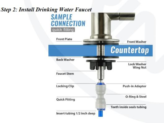
If your kitchen sink does not have an existing 1/2" faucet hole, you can either drill a hole (Refer to *How to drill a Hole on Sink or Counter-top*), or use the enclosed faucet bracket (Refer to *Installing the Faucet Bracket*).
