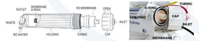
Step 6. a. Disconnect the tubing from the quick-fitting connection on the membrane cap.Step 6. b. Open the membrane housing cap. A thick rubber band can be slipped on the housing body for better grip.
