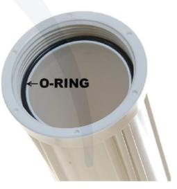
the housing on in a counter-clockwise direction by hand, and then use a housing wrench to tighten it up for about 1/4 - 1/2 turn. Do not overtighten, as this can cause leaks and make it difficult to unscrew the housing when replacing filters.
