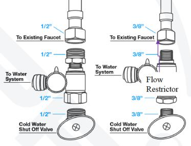
The included bushing can be threaded on either side of the Feed Water Adapter to fit the configuration of both 3/8" COMP and 1/2" NPT.
